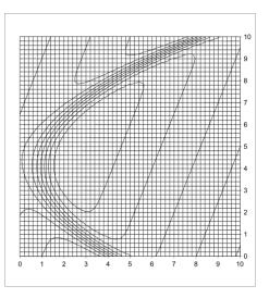
contours represent the economic risk (probability of an event times the cost of the event). The minimum is at the toe. The horizontal axis, x1, represents the dam height. The vertical axis, x2, is the setpoint portion of full.
