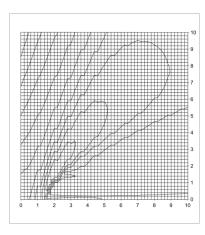
There are three difficulties with this problem. First, the steep valley causes difficulty for some gradient-based optimizers. Second, the nearly flat plane in the lower right can lead to premature convergence. Third, the surface has slope discontinuities due to the time discretization of the simulation. These can be made more visible with a larger simulation time increment, and appear as irregularities on the contour lines on the left. Ideally, the function is continuous in time, and
