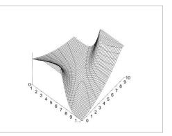
The minimum is at about x1=8, x2=2 in the near valley. The function is relatively well behaved, and even though it represents a sum of squared deviations, it is not a quadratic shape. Further, trial solutions in the far portion of the valley send the solution toward infinity (x1=- $\infty$ , x2=+ $\infty$ ).
