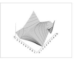
multiple runs will lead to multiple ending points that trace the valley bottom. The surface has another minimum in a valley in the upper right, and a well behaved local minimum up on the hill in the far right. Both the Parameter Correlation and the ARMA Regression function have a similar feature. This exaggerates it, and has a very simple formulation.
