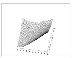
distance3 = Sqr((xb - x2)  $^2$  + (yb - y2)  $^2$ ) timetravel = distance1 / v1 + distance2 / v2 + distance3 / v3 f\_of\_x = (timetravel - 12) \* 10 / (32 - 12)
