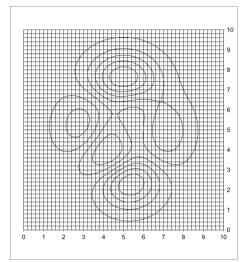
at (4,4), down the valley at (5.5,5.5), over the side of the mountain at (7,7) and down to (9,9). Alternately, if the path goes from (1,1) to (5,3) it stays on level ground. Then to (7, 6.5) it does not go into the middle valley, and only rises to the lowest point (the pass) between the two upper-right mountains. While the projection of the curved path might be longer, it does not rise or fall, and is actually a shorter path.
