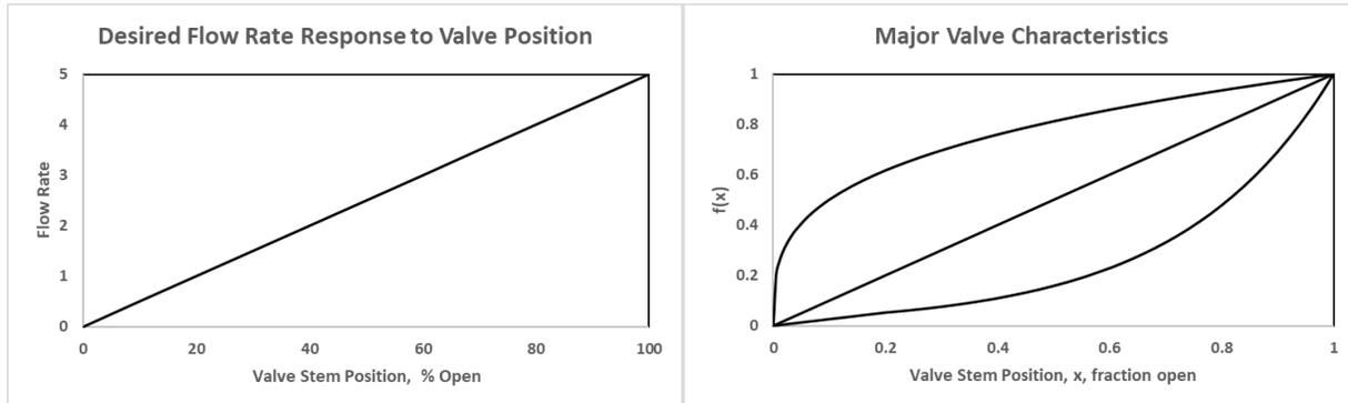
Figures 1 & 2. 1) A linear flow rate response, and 2) three categories of valve characteristics
