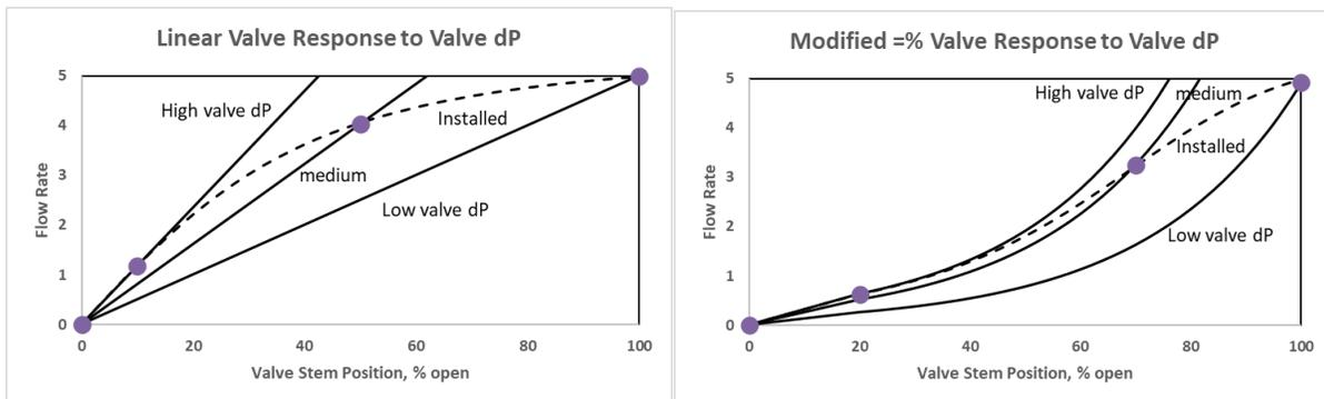
Figures 3 & 4. The installed characteristic of 3) a linear valve, and 4) and equal-percent valve.
